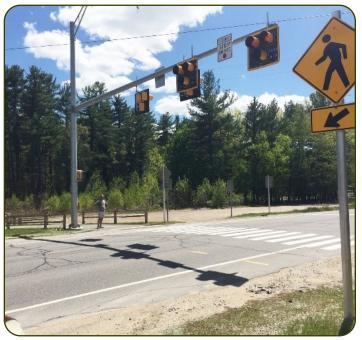
Figure 14: Trailhead access crossing with PHB. Source: FHWA
