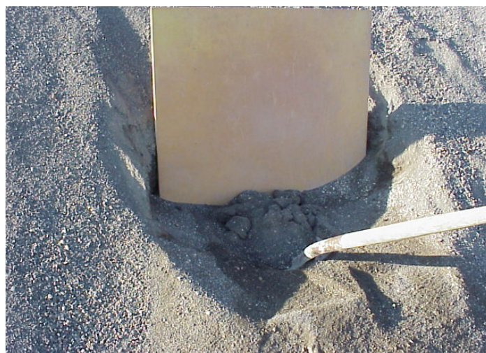
Exhibit 3-14 Proper Use of Shield for Sampling
