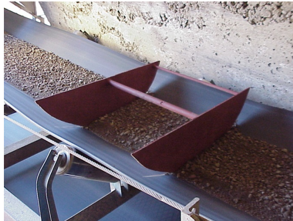
Exhibit 3-18 Proper Device for Belt Sampling
