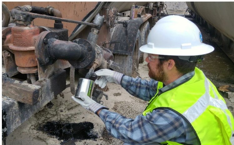
Exhibit 4-26 Sampling Asphalt Binder
