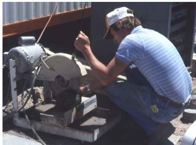
Exhibit 4-34 Sawing to Separate Pavement Layers
